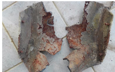
Burned out cast-iron baffle plate, about three years old. The owners used softwood, which has a bigger fuel load than hardwood, causing flames to be too close to the baffle plate, which caused it to warp and fail—the middle part is missing.
