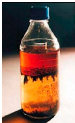
Microbial mat at the fuel/water interface of contaminated diesel
