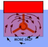
This happens under the counter of the boat, and because the water is flowing faster in the same direction as the blades, the blades have less 'bite' on it. Under the boat there is more room so the water flows slower and the blades are able to push against it and drive the stern sideways. If the bottom of the canal is close the flow is again confined, speeding up and balancing the effect under the counter.
