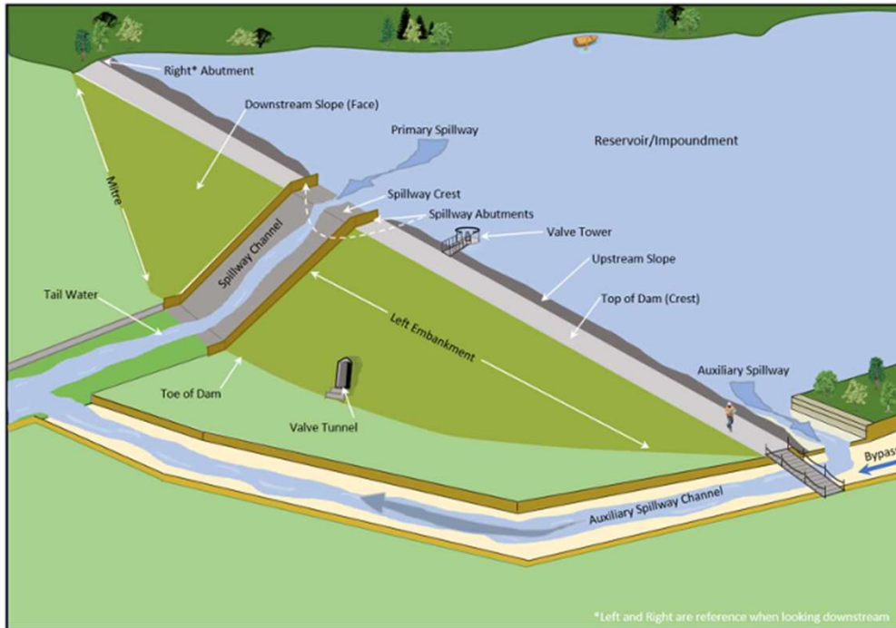
Figure 1 - Reservoir typical arrangement and terminology
